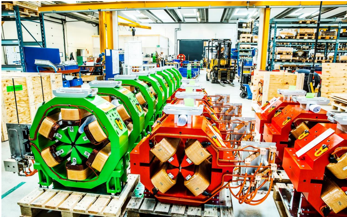
Figure 3. Hexapole (green) and Quadrupole (red) magnets to the new EBS storage ring at the ESRF (figure from https://www.danfysik.com/ ).
